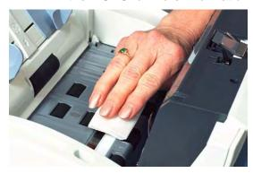
2. Wipe the upper and lower imaging guides with an almost dry Staticide wipe to remove any streaks.
